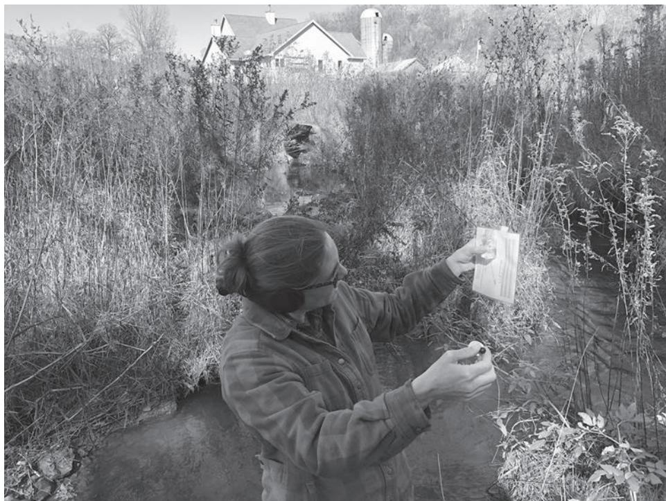
Left: Bethany Emond Storm measuring dissolved oxygen (DO) in her stream using a Hach test. If a sudden drop in DO is found, it could identify an acute issue with the stream that would require notification to the DNR.
